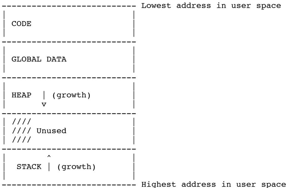
1. The code region contains the machine-language version of the program. This is typically loaded at program startup, and is not changed during program execution. (Often, this region of memory is mapped "read-only" during program execution.
