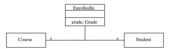
(Note the use of the three sets of lines in the box representing the association class, to make it crystal clear that this is a class.)
