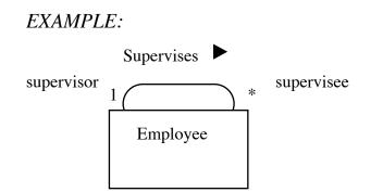
Note: Care must be used in drawing a diagram to distinguish between the name of an association and role names. The latter should be drawn near the end of the association line; the former far enough from the ends to be clear that it is not a role.
