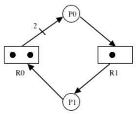
3. On the other hand, the presence of a cycle in the graph does not necessarily indicate a deadlock if there is some process not part of the cycle that can release a resource that breaks up the deadlock.
