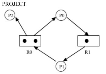
Now, though P0 and P1 are currently deadlock, the deadlock will be broken if P2 releases its instance of R0
